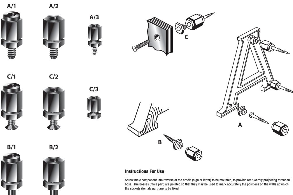
The sockets (female part) are then screwed to the wall or support so as to be rotatable on the screws and are then screwed around the mounted bosses (male part) until tight.
