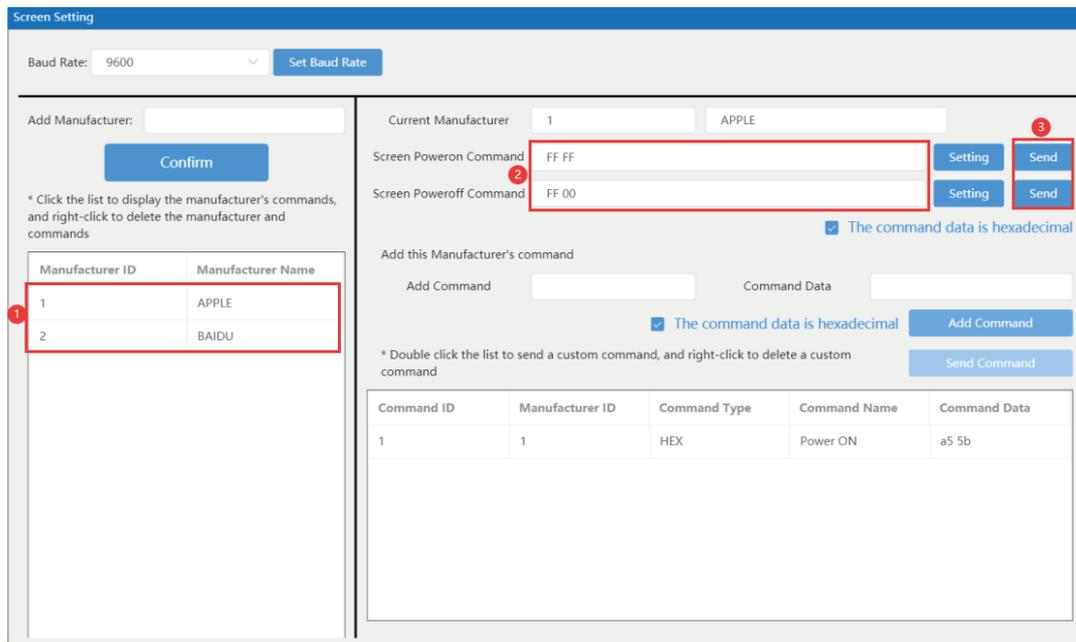
**Method 2:** Click “Screen Poweron / Screen Poweroff” on the Main Function interface to send the manufacturer power on/off command that is set for the last time.
