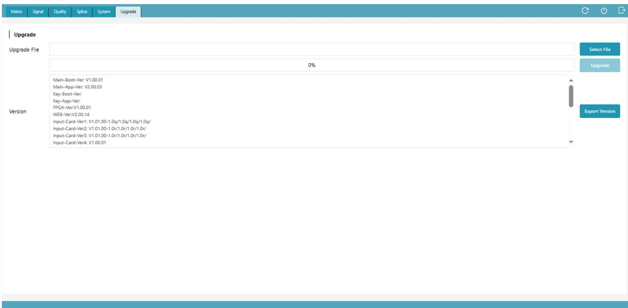
Click “Select File” to select the upgrade file, then click “Upgrade” to start the system upgrade. After the progress bar reaches 100%, the upgrade is successful, and the device will reboot automatically.
