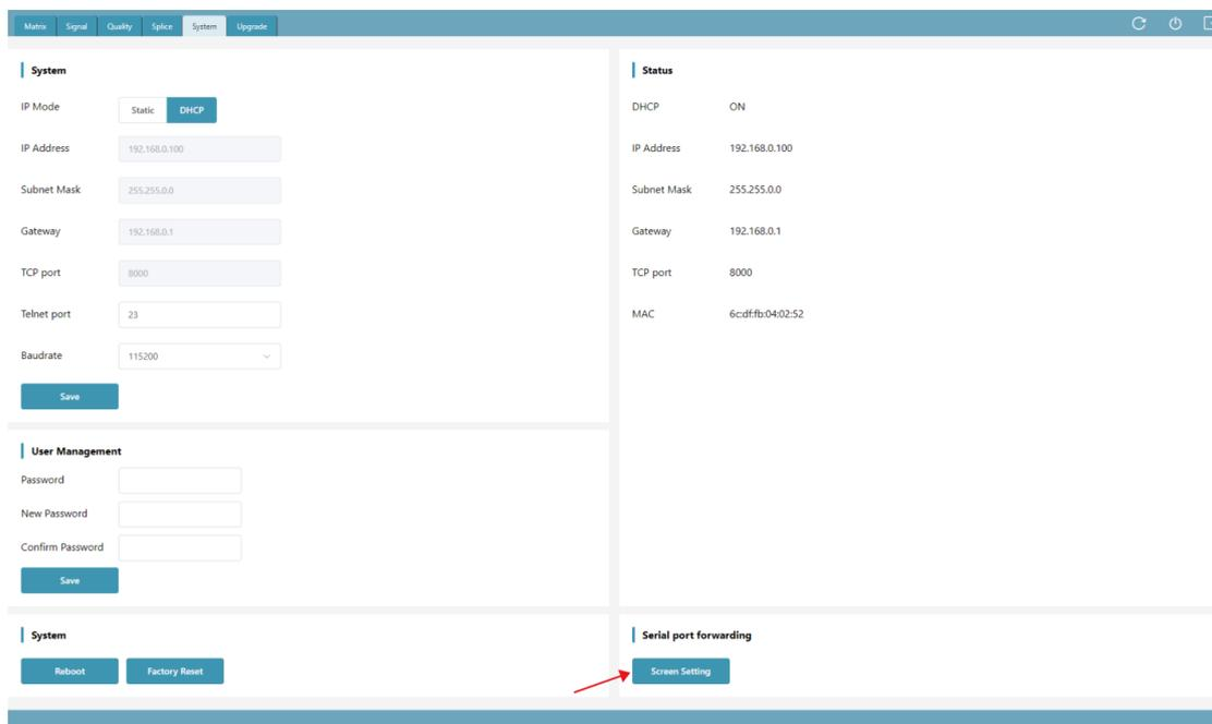
Click “Screen Setting” to enter the Screen Setting page, as shown in the figure below. You can add the command (ASCII/HEX) for the manufacture and select the baud rate, then click “Send” to send commands through the external serial port.
