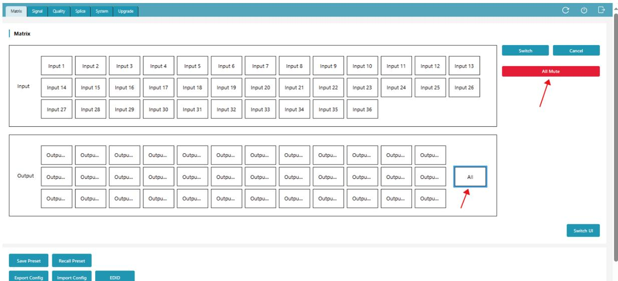
③ Turn off the output: As shown in the above figures, double-click an output port, then click “All Mute” to turn off the audio and video output of the selected output port; double-click “All”, then click “All Mute” to turn off the outputs of all output channels.
