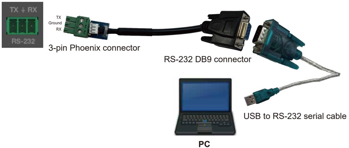
**Step 2.** Check “COM” on the Connection page, and select the corresponding COM Port and Baudrate (default Baudrate: 115200). Then click “Confirm” to connect the device.
