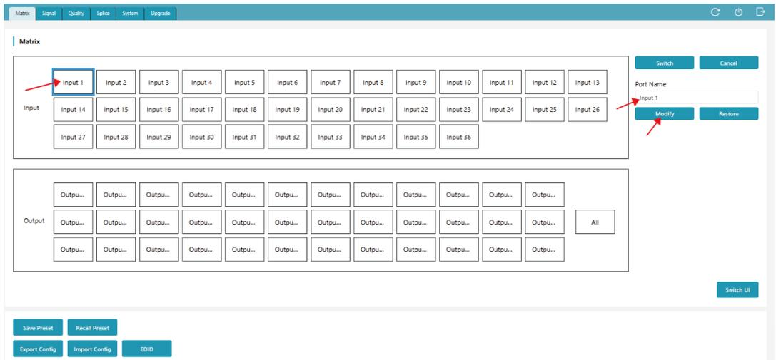
① Modify the name: As shown in the above figure, double-click the input/output port, then edit the name in the input box of "Port Name" (The name supports numbers, uppercase and lowercase letters and spaces, not all spaces. The maximum length is 32 English characters or 16 Chinese characters). And then click "Modify" to complete the name modification.
