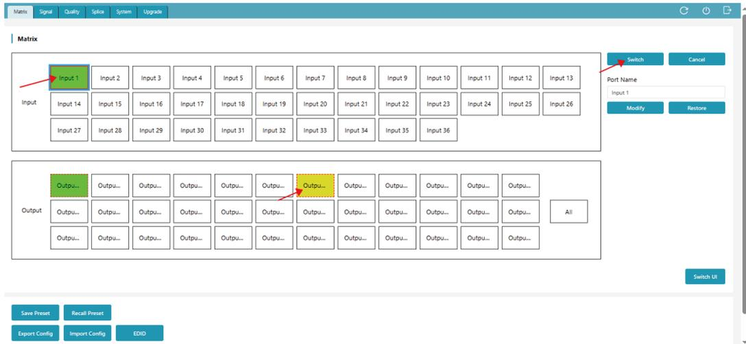
② Switch matrix correspondence: As shown in the above figure, click an input channel, and then click an output channel or click “All” (the selected output channel will turn to yellow), finally click "Switch" to take effect. After switching is completed, the output channel will turn to green.
