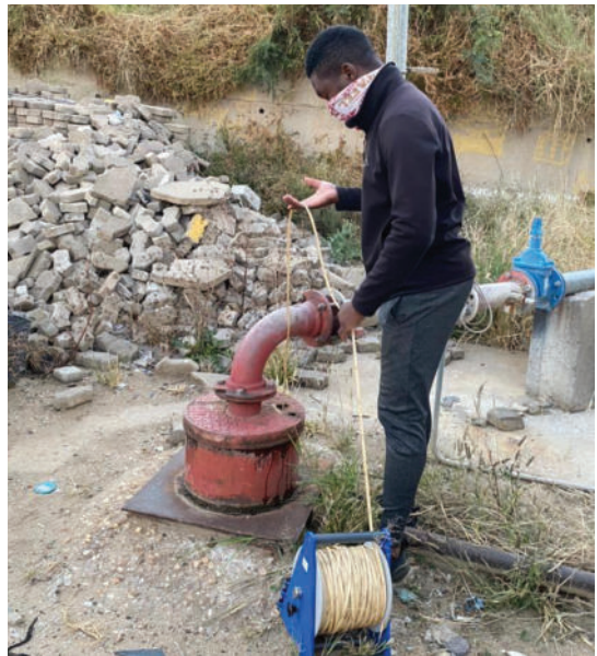
Figure 1: Demonstration of groundwater level measurements
