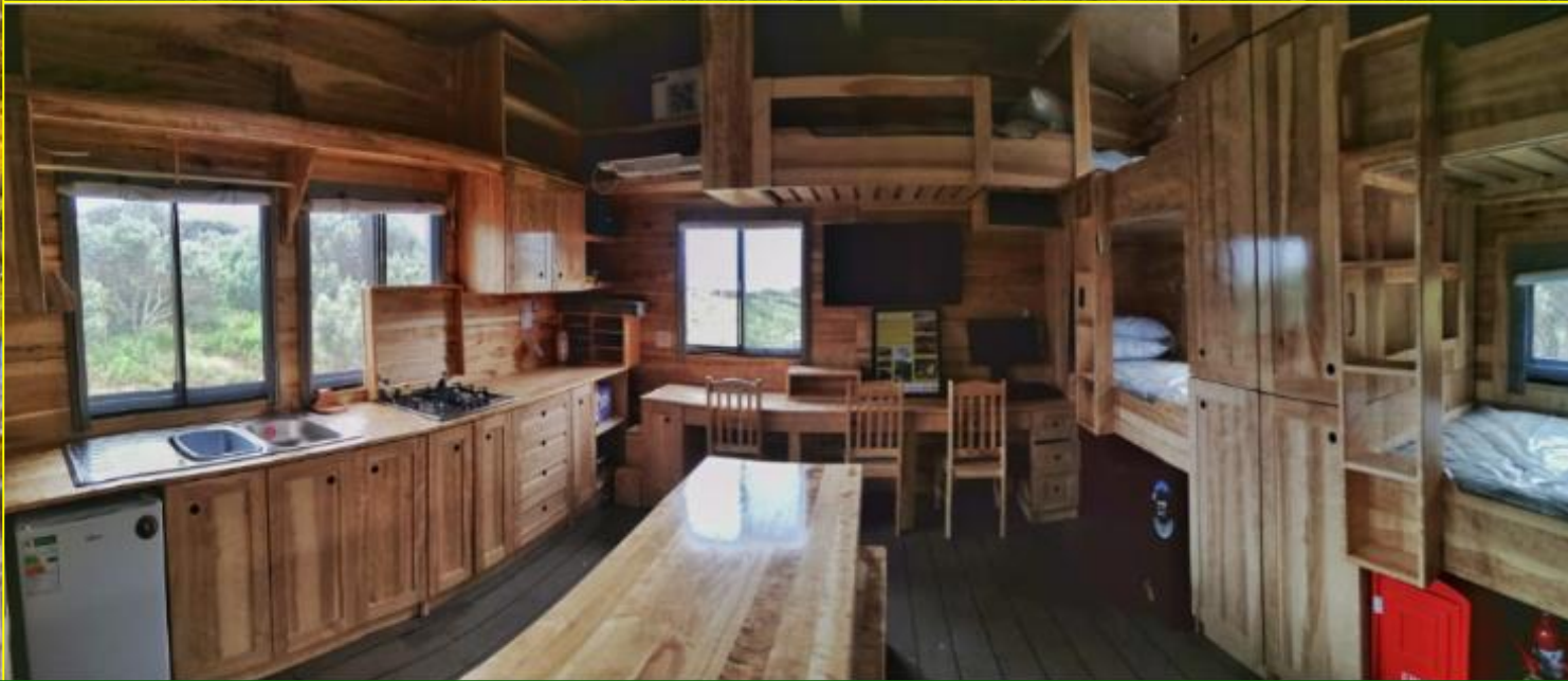
An Emergency Hut was built on Gough Island (which can sleep ten people), with wood-plastic composite cladding, and furniture and fittings from invasive poplars.
