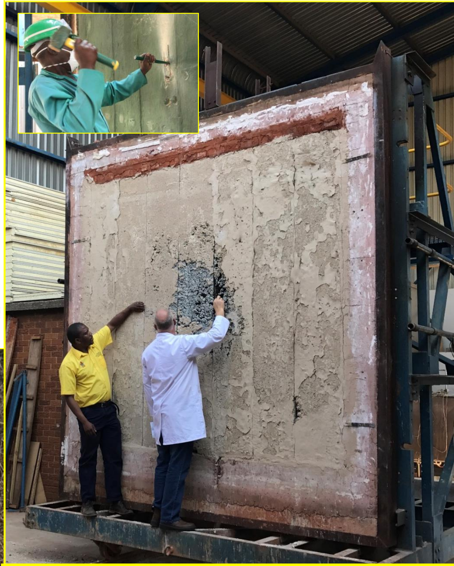
Cross-cut sample of 200mm Light House wall after exposure to 1 100 C furnace for 3 hours, 70% chipped gum trees
